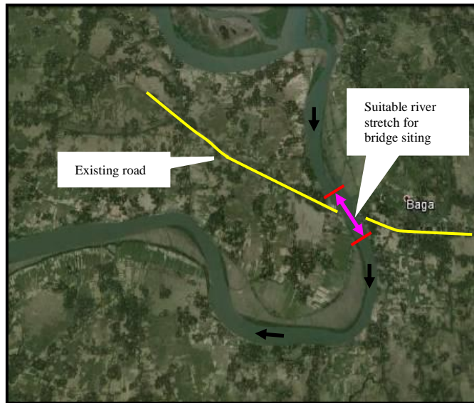
Fig. 3. Suitable river stretch for siting of the bridge
