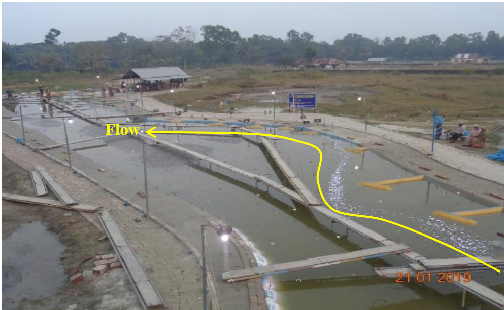
Fig. 3. Flow diversion by the groynes during model run (T6)
