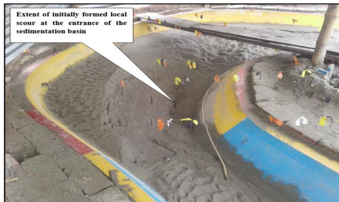
Fig 9. Extent of initially formed local scour at the entrance
