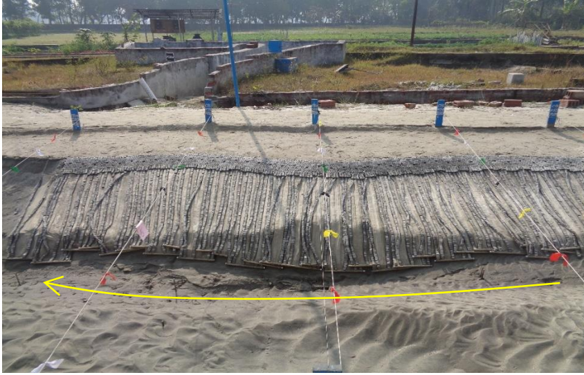
Fig.3. Scour pattern around CBM after run (T14) in the model
