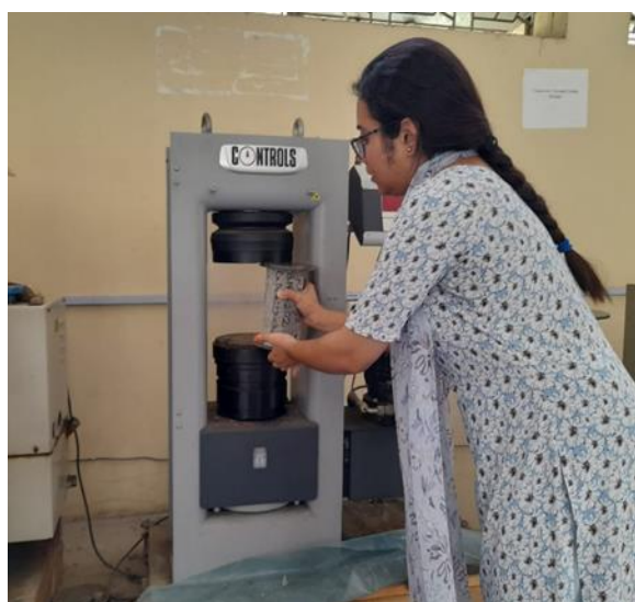
Figure: Marzia Sultana Shefa, operating Concrete Crushing Machine for measuring compressive strength of the blocks at the Material Testing and Quality Control lab
