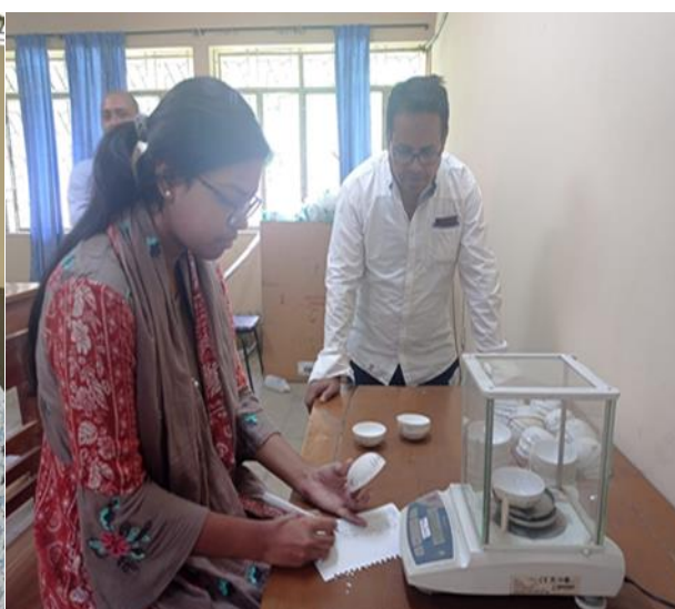
Figure: Suparna Sarker, weighing the amount of suspended sediment for determining sediment concentration at the Sediment lab
