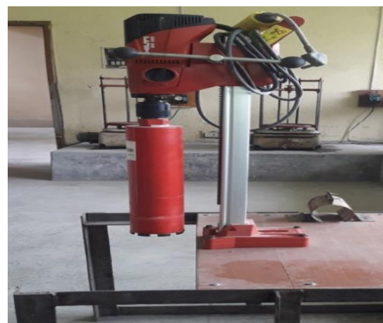
Recently purchased equipment (supported by IDCB Project, Phase-II) for Concrete and Material Testing Laboratory: Concrete crushing machine (Controls, Italy) (left) and Core cutter machine (Hilti, Switzerland) (right) used for cutting concrete block and extract core.
