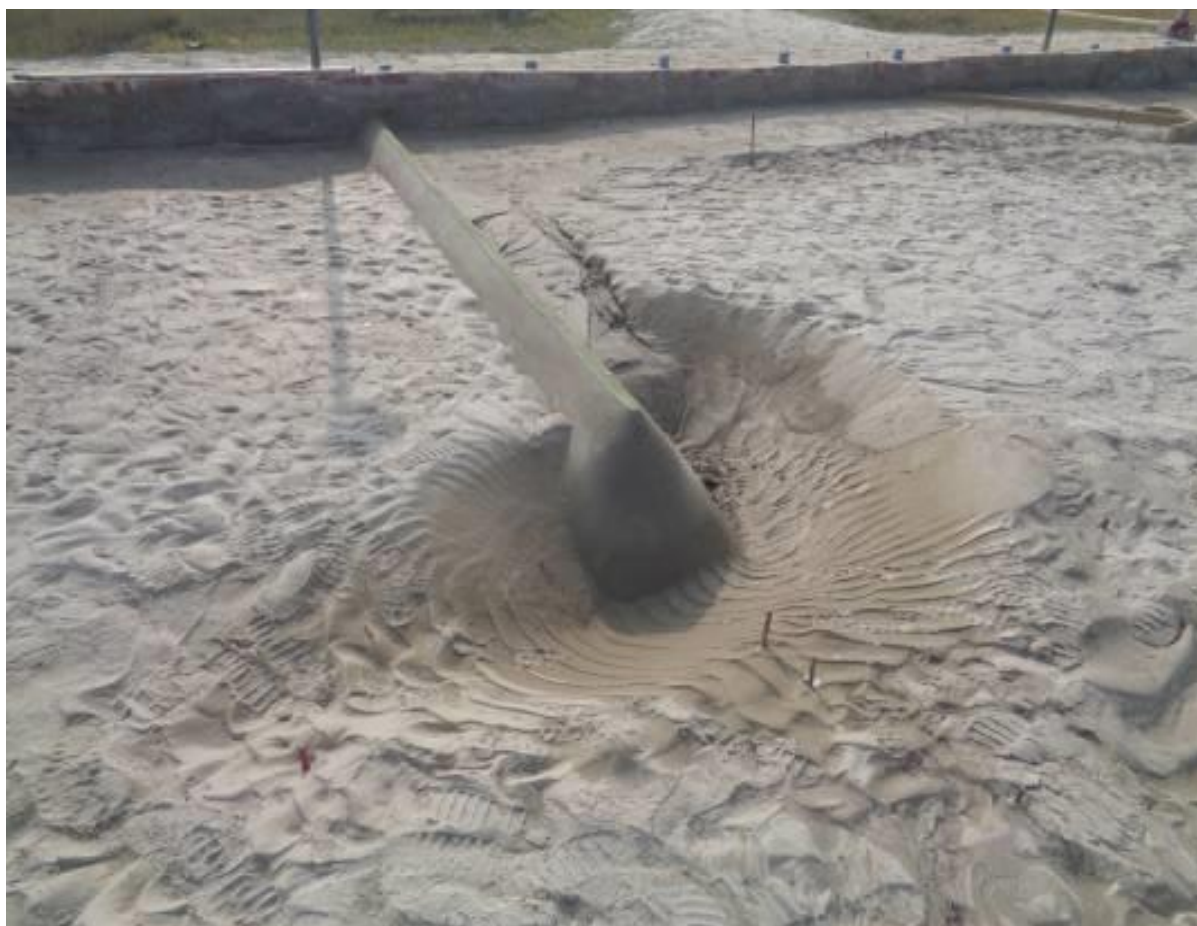
Local Scour around temporary cross-bar in the Teesta Barrage Model
