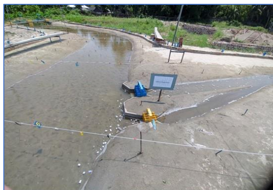
Flow through the Upper and Lower Karatoa River Model
