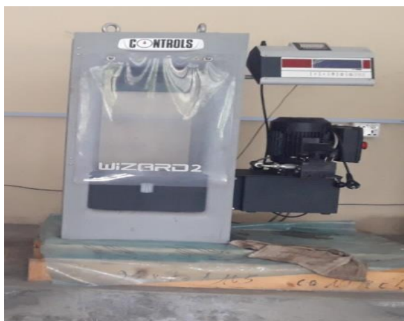
Recently purchased equipment (supported by IDCB Project, Phase-II) for Concrete and Material Testing Laboratory: Concrete crushing machine (Controls, Italy) (left) and Core cutter machine (Hilti, Switzerland) (right) used for cutting concrete block and extract core.
