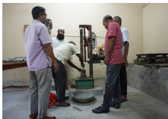
Sample preparation for Limit test of disturbed soil samples (left) Compaction testing Electro Mechanical Instrument (right)
