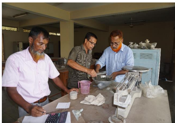
Sample preparation for Limit test of disturbed soil samples (left) Compaction testing Electro Mechanical Instrument (right)
