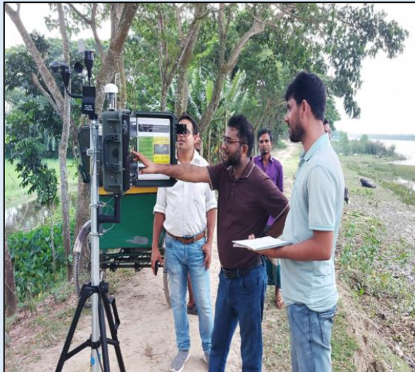
Recently RRI is using Portable Air Monitoring System with rain gauge (HAZ SCANNER, Model: HIM-6000) for Environmental Monitoring and EIA study.
