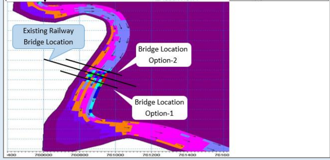
Figure: Velocity fields at and in the vicinity of the likely bridge locations (option-1 & 2) for 50-years return period disc
